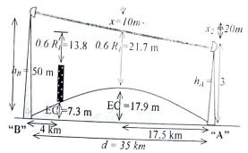
Very clear the existing obstacle has no effect and the dominant height is the mid way height. Since site "B" tower is 50 m height and the effective obstacle height is 40 m at mid way, thus the tower height at sit "A" is 30 m.
